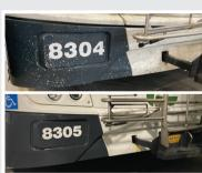
"As Nano-Clear® has significantly reduced the number of stone chips to the front bumper, and has proven to be a more resilient stone quard, Engineering recommends that future bus deliveries, and buses that go out for refurbishment have the NCI stone guard applied."
