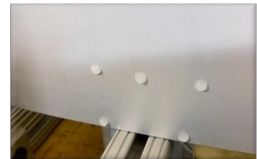
Sample of Ice De-bonding Test on Aluminum Substrate (NCI +MA +EC: 40 seconds)
