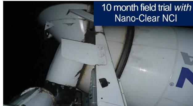
Even sticky concrete dust releases easily from Nano-Clear® NCI.
