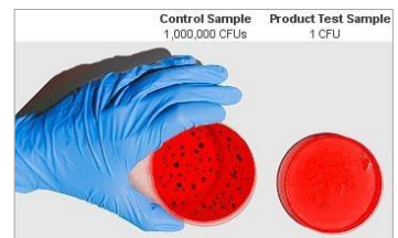
Sample Log Reduction Test (Comparing CFU (Colony Forming Units), Before & After)
